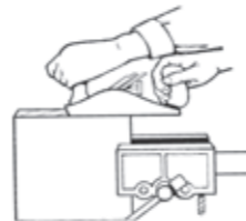
Fig 2 Plane ends with a bench plane
