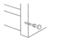
Fig 20 Screw and cap with timber plug
