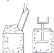
Fig 4 Setting the posts.
