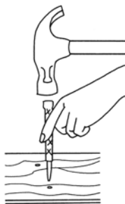
Fig 13 Send the nails below the timber surface with a nail punch.
