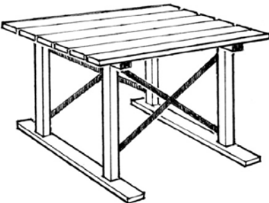
Typical tank stand
