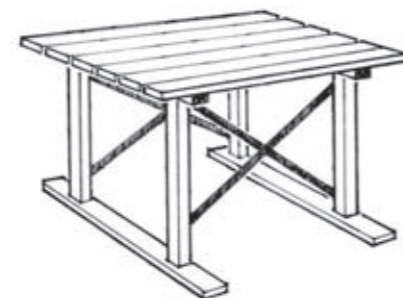
Typical tank stand
