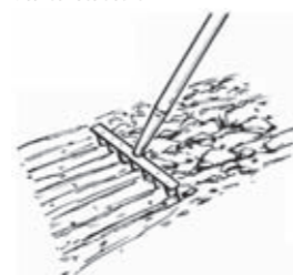
Clear surface debris
