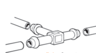
Fig 4 T-connectors for sharp bends
