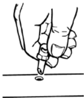
Fig 7 Push dripper or spray heads into punched hole in the tubing or onto riser tubes
