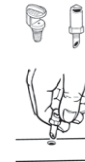
Fig 7 Push dripper or spray heads into punched hole in the tubing or onto riser tubes
