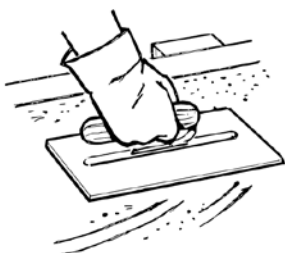
Fig 11 Smooth the surface with a steel trowel.
