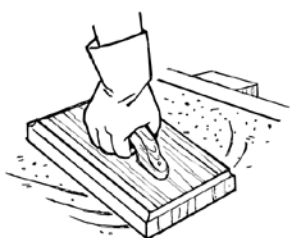
Fig 12 Use a wooden float for non-skid surface.
